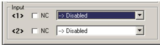
In the inputs area of the REM n board you must program the supplementary command and control devices (e.g. safety buttons, sensitive footboards, alarms etc.) that will be connected to the REM and act on any one of the RBM84 and REM outputs.
